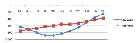
•FASTENER TK reads 10% short off metal (or on non metal surface). It can be applied for BOTH metal and off metal application.
