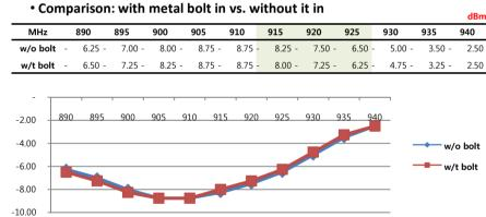
•FASTENER TK reads same, regardless of whether it is fastened with metal bolt in two holes (located on center of both ends) or not. Stainless steel M4 bolt with round head is best fit for FASTENER.
