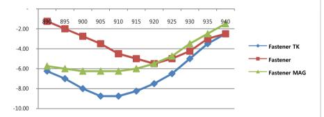
•FASTENER TK reads up to 12.0 meters on metal, almost double of FASTENER and FASTENER MAG. It's one of best performing among 4mm thick metal tags with most stable and consistent read, as its slow and gentle slope of sensitivity curve shows.
